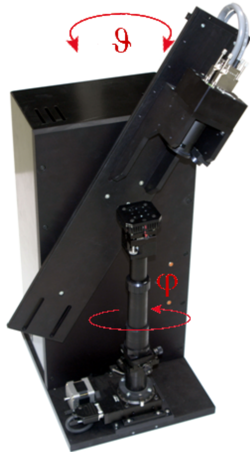
Figure 2.12.: TechnoTeam LED goniometer [www03]
