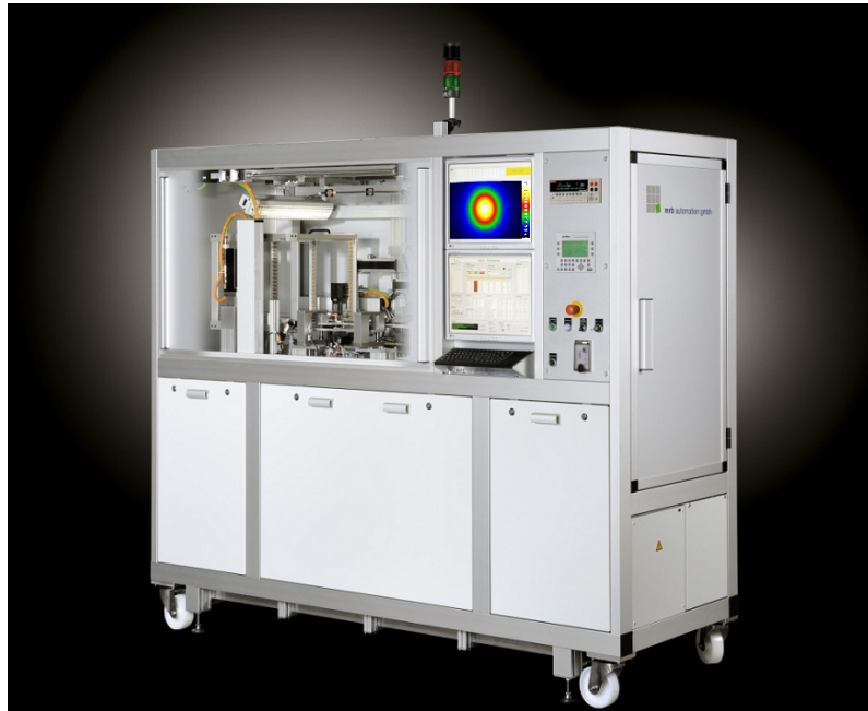
Figure 4.4.: Automatic adjuster for adjusting cold light reflector lamps
