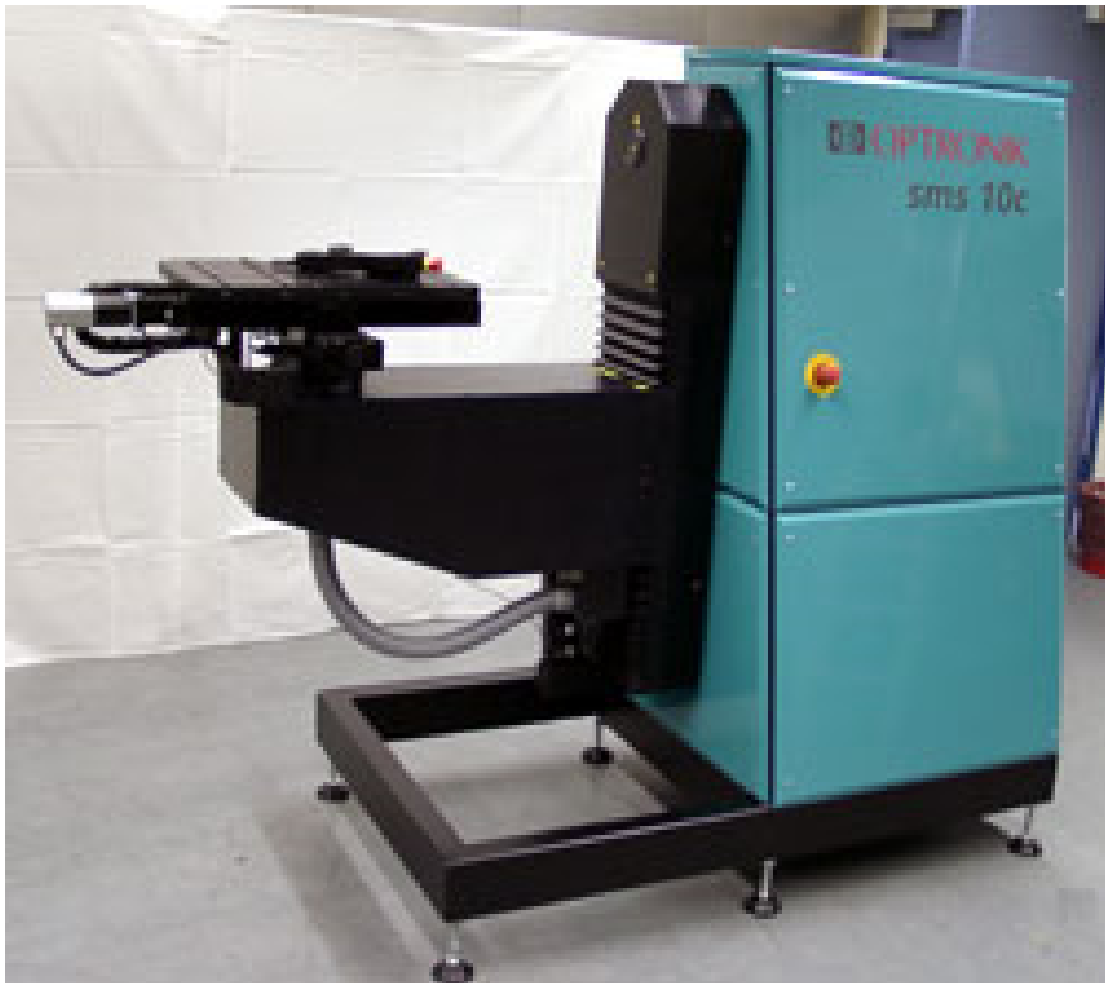
Figure 2.2.: Optronik SMS10C luminaire turning device; front view [www04]
