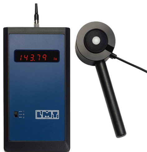
Figure 1.10.: LMT Pocket Lux 2; manual lux meter [ www02 ]
