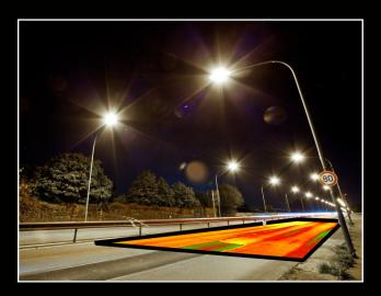
According to the measurement methods described in EN 13201-4, measurements with an **LMK** are considered to be the current technological state of the art. The **LMK** is used here to record a high-resolution measurement image of the road
