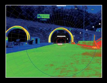
For this measurement task, the required measurement data are the average luminance of the roadway in the tunnel portal (entrance section) and the surroundings of the entrance portal in a 20° environment. The alignment of the **LIVIK** is made easy
