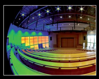
There is a distinction between daylight glare and artificial light glare. Depending on the lighting situation and visual task, different metrics are introduced for evaluating glare (UGR, DGI, DGP, etc.). The **LIMK** has the metrological prerequisites
