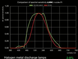
Integral spectral matching error in % for lamp
