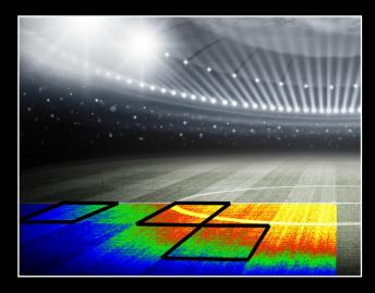
Determination of glare characteristics of artificial outdoor lighting systems, e.g. of sports facilities or outdoor advertising. These include the maximum tolerable luminance (according to LAI), the vertical illuminance or the equivalent veiling luminance.
