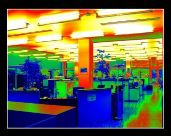
The photometric evaluation, in accordance with parts of EN 12464-1 is easy with the **LMK**. The measurement of luminance and visually perceived contrasts serves as a measure of the ergonomics of visual tasks.
