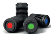
Multi-Color calibration with different L^* standards.
